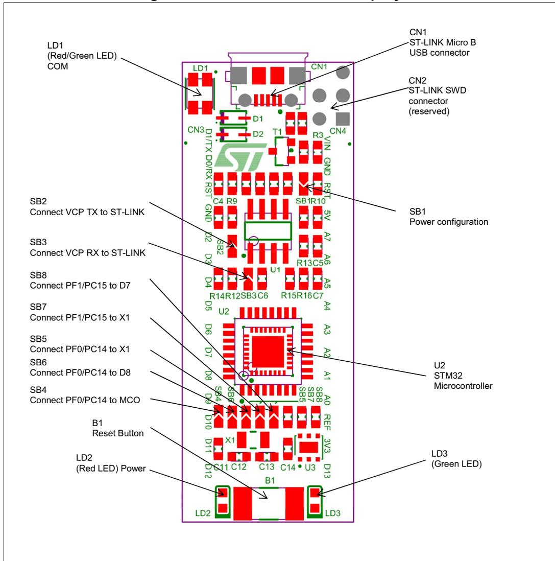
Figure 4. STM32 Nucleo-32 board bottom layout
