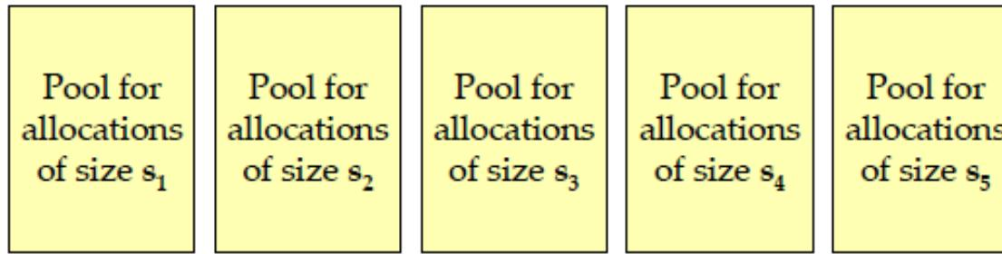
$n$ -byte requests handled by first pool with size  $\geq n$  and non-null free list.
