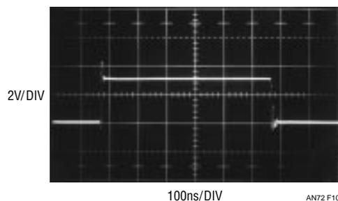
**Figure 10. Transition Instabilities Due to No Ground Plane**
