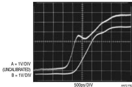
**Figure 82. Pulse Stretcher Waveforms in 3.9GHz Bandpass Show 650ps Output Rise and Delay Times (Trace B). Nonlinear Loading Causes Input Transition Aberration (Trace A), but Is Not Deleterious. Trace Granularity Derives from Sampling Oscilloscope Operation**
