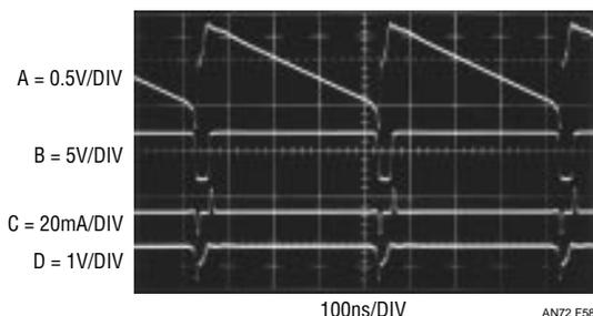
**Figure 58. Precision 10MHz Voltage-to-Frequency's Operating Waveforms. LT1122 Integrator Is Completely Reset in 60ns**
