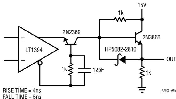
Figure A2. Level Shift Has Noninverting Voltage Gain
