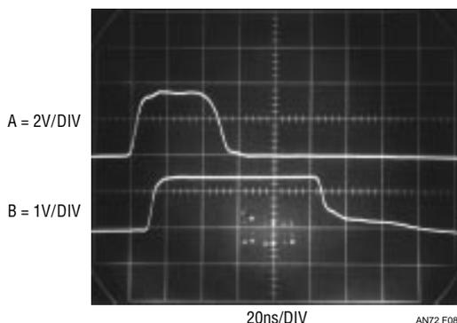
Figure 8. Overdriven FET Probe Causes Delayed, Tailing Response
