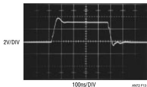
**Figure 13. Excessive Load Capacitance Forces Edge Distortion**
