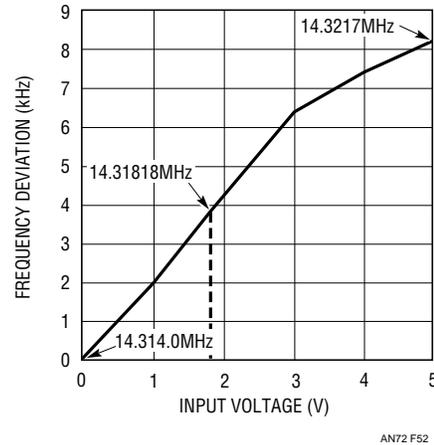
**Figure 52. Control Voltage vs Output Frequency for Figure 51. Tuning Deviation from Center Frequency Exceeds  $\pm 240$ ppm**
