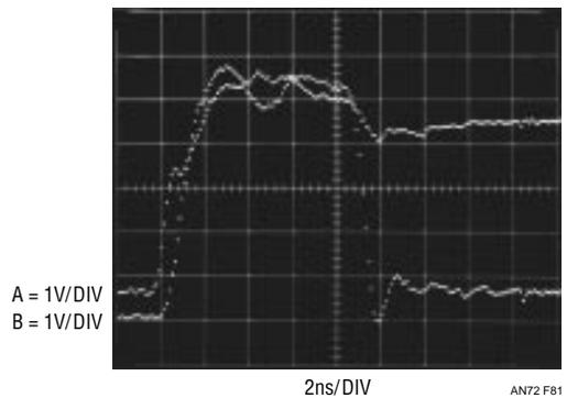
**Figure 81. Pulse Stretcher's Input-Output Relationship in a 3.9GHz Bandpass. Output Amplitude Drops When Input Decays, but Logic Level Is Maintained. Sampling Oscilloscope Display Is a Series of Dots**
