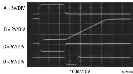
**Figure 70. Voltage-Controlled Delay's Waveforms. Programming Voltage Determines Delay Between Input (Trace A) Falling Edge and Output (Trace D) Rising Edge. High Linearity Timing Ramp (Trace B) Permits 1ns Accuracy and 100ps Repeatability**
