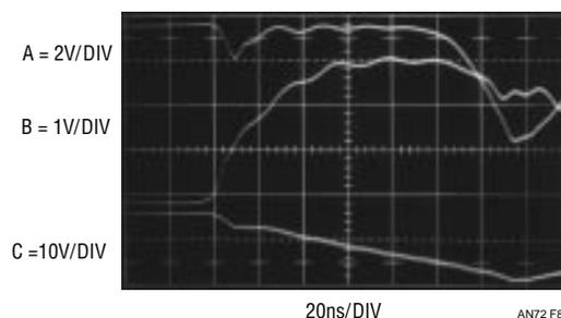
**Figure 85. Detail of Protection Circuits Behavior. Output Amplitude Excursion (Trace A) Triggers Comparator (Trace B), Resulting Gate Drive Removal (Trace C). Overvoltage is Arrested in 20ns, Complete Shutdown Requires 150ns**
