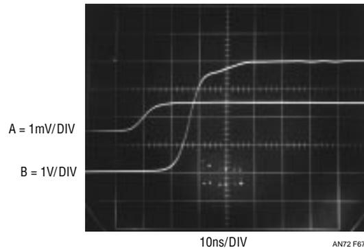
**Figure 67. Parallel Path Comparator Shows 18ns Response (Trace B) to  $500\mu\text{V}$  Overdrive (Trace A)**
