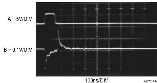
Figure 44. Response of 10 $\mu$ F Tantalum Capacitor
